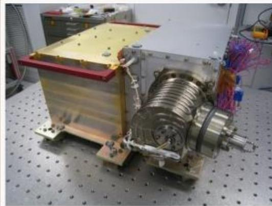
The NGIMS instrument measures the composition and isotopes of thermal neutrals and ions in the Martian atmosphere. (Courtesy NASA/GSFC)
